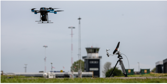
Fig. 2: AUT in the measurement environment, with the UAS-APE approaching it.
