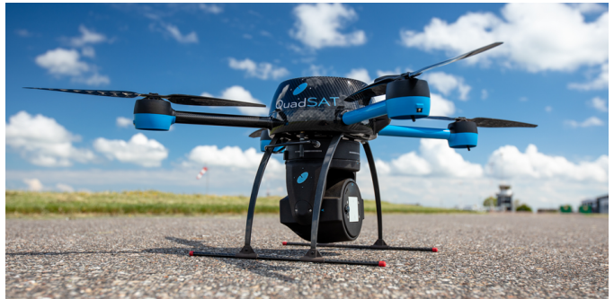
Fig. 1: QuadSAT’s compact UAS-APE. The compact gimballed remote source antenna can be seen situated under the drone.
