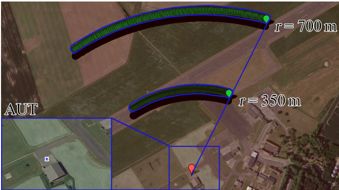
Fig. 3: QuadSAT's outdoor range and waypoints of the scanned positions. (Credits: Google Maps)
